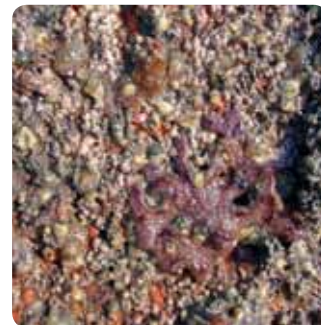
Various fouling species found on a test panel without anti-fouling coating after a 12-month exposure.
