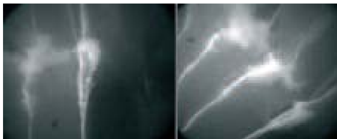
Figure 6 - Propeller cavitation (Courtesy EROCAV)
