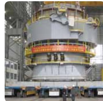
Pedestal assembled with slewing system sent from the workshop by a jacking platform.
